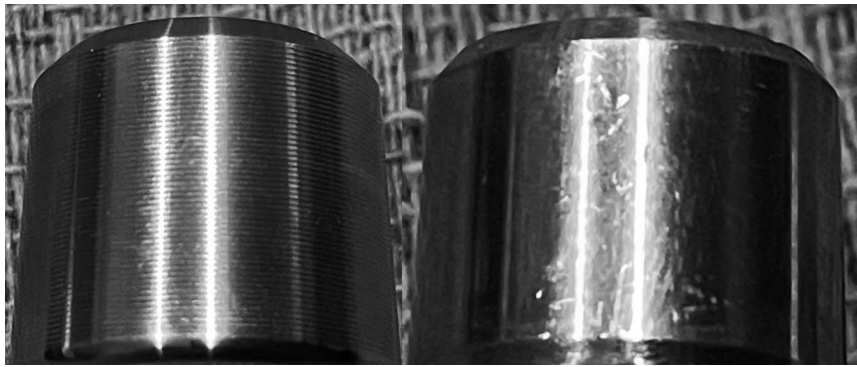
Photograph of a grooved trunnion on the left and a smooth trunnion on the right.
