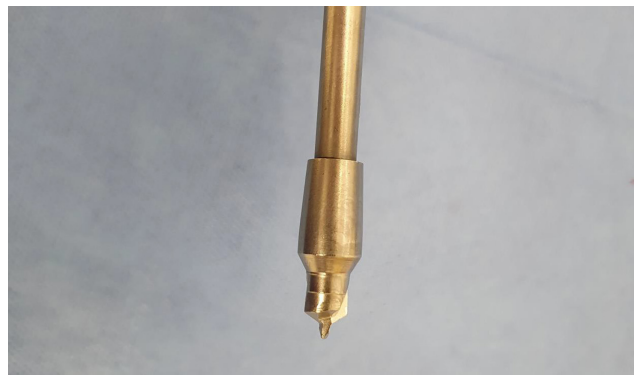
Figure 4 Example of the drill utilized for acetabulum cement hole creation.
